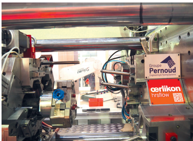
Fig. 9. Two-component mold from Groupe Pernoud with two different hot runner systems from Oerlikon HRSflow, which permits automatic exchange between three product variants without dismounting the mold.
